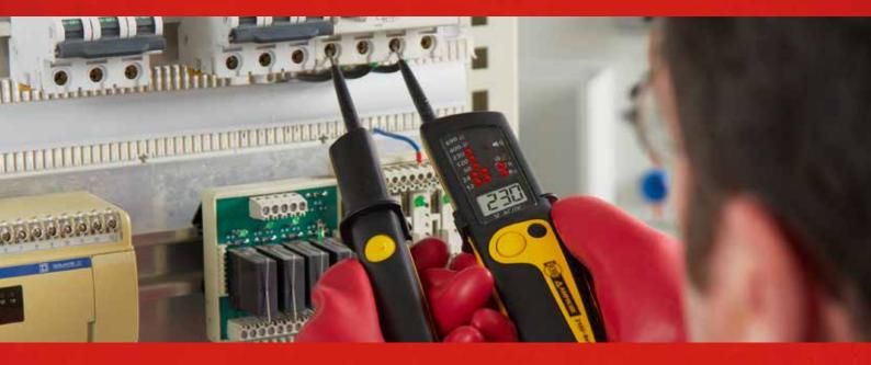
The Beha-Amprobe 2100 series are rugged, easy-to-use two pole voltage testers for voltage and continuity checks. Built tough for use in industrial and commercial environments.
